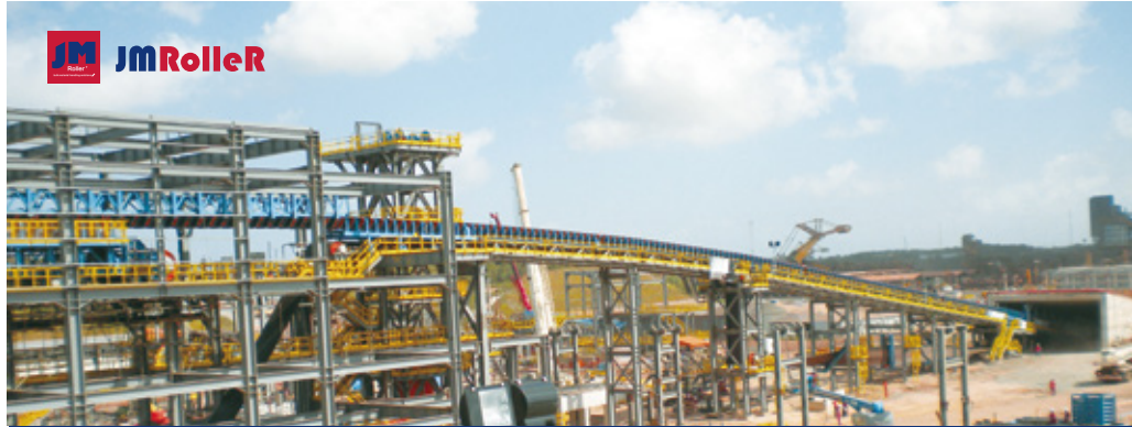
Belt Conveyor Machine
