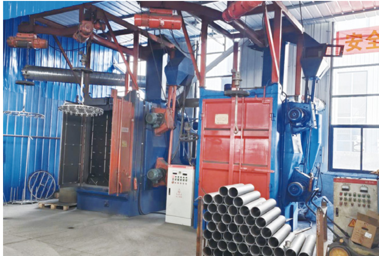
2 Rust Removing Machine
